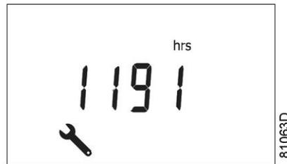
This screen shows the unit used <hrs> (or <x1000 hrs>) and the value <1191>. In the example shown, the compressor has run 1191 hours since the previous service (i.e. the last time the timer was reset).
