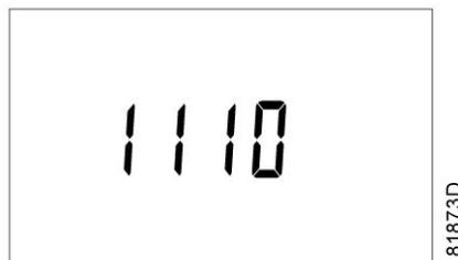
The screen shows (from left to right) the status of the remote start/stop switch, the electronic condensate drain contact and the flow switch.
