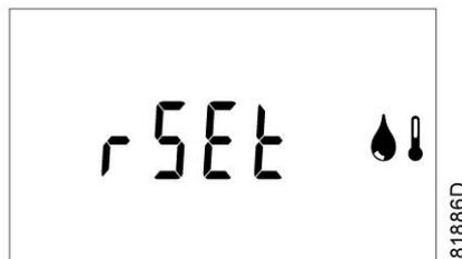
Press Enter button (13): the programmed value starts blinking. To change, use the Scroll buttons (12). Press Enter button (13) to modify.
